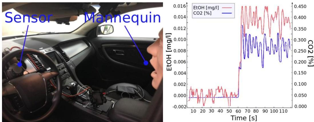
**Figure 5. (a) Experimental setup in a vehicle compartment for investigations of the feasibility of unobtrusive testing. The sensor was located at the steering wheel and gas pulses were generated from a mannequin 65 cm from the sensor. (b) Recording of ten consecutive gas pulses starting at 60 seconds. The gas pulses contained 0.4 mg/l ethanol and 5 vol% CO<sub>2</sub>, and had a total volume of 0.5 l during 2 sec, which is representative of human breathing at rest.**
