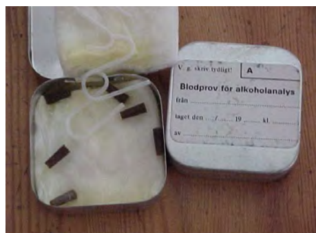
SMALL METAL CONTAINERS USED TO SEND SIX BLOOD CAPILLARIES TO A CENTRAL LABORATORY FOR ANALYSIS.
